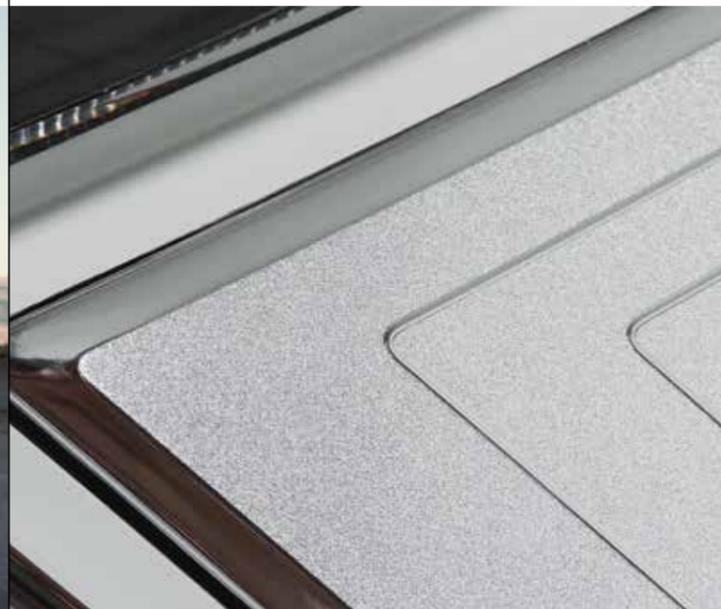
⊖ ⊕ Attention to detail: design contours on the Audi A6's headlamp are emphasised by lines that are embedded in a finely lasered structure.
